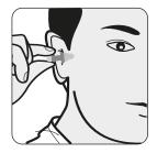
2. Grip the plastic handle of the Rocket plug and slide the plug into the ear canal. Rotating the plug slightly whilst inserting may help.
