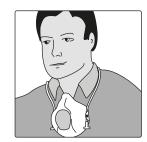
5. Unbuckle to take off. During work breaks open the buckles and let the mask hang around the neck.
