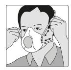
Ensure respirator fits secure and comfortable. To fasten respirator pull strap at either side of the buckle.
