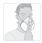
Close the vents of the exhalation valve by pressing down the flexible valve cover and breathe out slowly. If no air escapes between facepiece and face, a proper sealing fit is achieved. If air escapes, adjust the position of the mask on the face or adjust the tension of the straps. Repeat this check until a seal is achieved. If a secure seal cannot be achieved, do not enter any contaminated area. See your supervisor.
