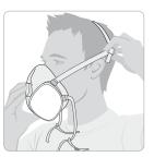
Place the respirator over the mouth and nose and fit the head straps as shown in the illustration.
