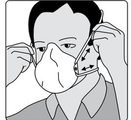
4. Adjust strap by pulling loop on strap.
