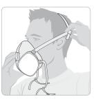
Place the respirator over the mouth and nose and fit the head straps as shown in the illustration.
